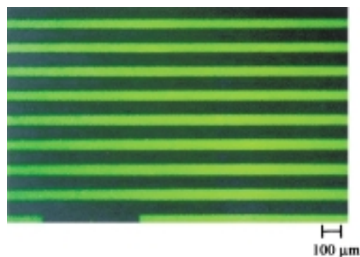
Figure 2. Fluorescent image patterns obtained with a 1.0- \mu m thick film containing copolymer 1 (77 wt %) and TPSHFA (23 wt %) on a silicon wafer after UV irradiation (360 nm) for 10 s ( 200 \text{ mJ cm}^{-2} ) through a photomask followed by heating at 120^\circ C for 1 min.
